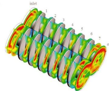
Archimedes screw mixer ensuring the copper particles are uniformly dispersed.
